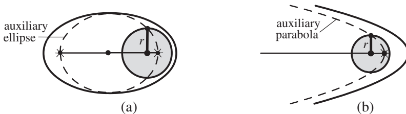
Figure 18. Auxiliary (dashed) conic used to construct a focal disk, for (a) an ellipse, and (b) a parabola.
